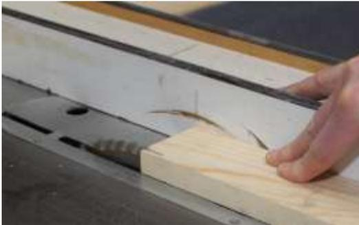
1. Cut the board a little wider than the final desired measurement.
