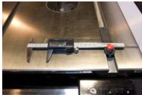
3. Place caliper and base assembly on the table saw close to the fence, extend depth probe to rest against the fence and set the calipers zero. If the calipers will not reach the fence, you can insert a board to fill the space. Since this is a relative measurement, size of the spacer is not critical.
