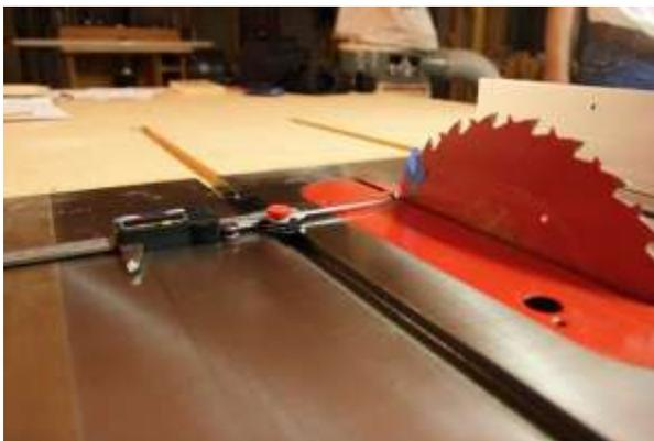
4. Retract the caliper, then rotate the blade so the mark is away from you, move caliper and Mitre Slot Base to the mark. Next, extend the caliper until it touches the blade. The reading on the caliper is the distance the blade is out of square.
