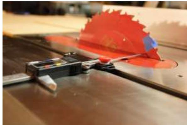
2. Place calipers in the Mitre Slot Base per figure on base. See instructions or tip on how to do this.
