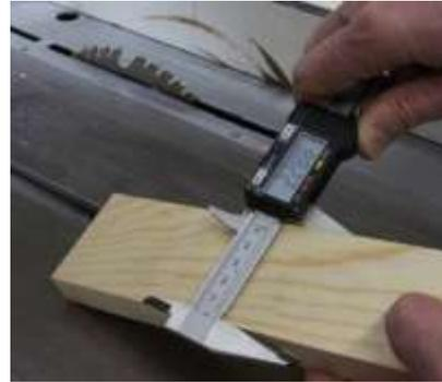
2. Measure board with the calipers to get an exact width. Note the difference to the desired width.
